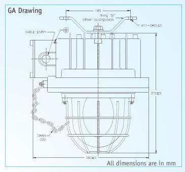
Flame Proof - Exd Type of protection Area Classification Zone 1 & 2 Gas Groups Group I, II A, II B & II C IS:2148-2004 (IEC 60079-1/2001) Apparatus Standard IS- 2206 Part I CIMFR Certificate No. CIMFR/TC/SR/H1113 CCE.BIS **Approvals** Temp Rating T6 **T6** T4 300 GLS 400 HPMV Wattage Rating 250 HPMV 500 GLS
